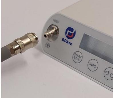
Fig. 2.3 Cuff connection of the ABPM devices
